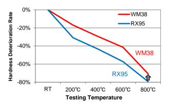
WM38's hardness deterioration rate at 800°C is improved about 10% in comparison with RX95.
