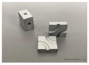
Two blocks on the right side is the cross sections of a left block. The hole has curved internal structures.
