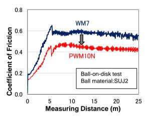
The coefficient of friction of PWM10N is lower than that of WM7.
